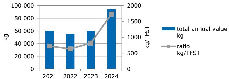
The increase in the consumption and waste of iron(III) chloride ( $\text{FeCl}_3$ ) is due to the significant increase in etching activity as well as the increasingly complex structures of textured belts.
